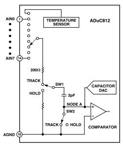
Figure 7. Internal ADC Structure
